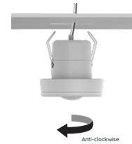
Rotate the lens anti-clockwise to remove from the case and clockwise to connect to the case
