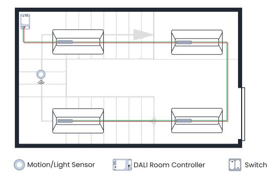
Stairwells require adequate brightness levels for efficient navigation and ensure safety. Utilizing motion and daylight sensors are effective ways to reduce energy consumption.
