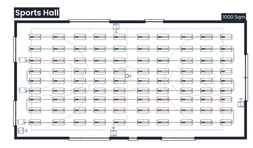
Motion/ Light Sensor DALI Room Controller Switch
