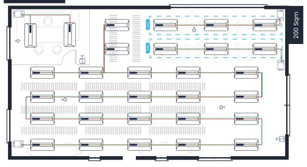
Motion/ Light Sensor DALI Room Controller Switch DZ: Daylight zone
