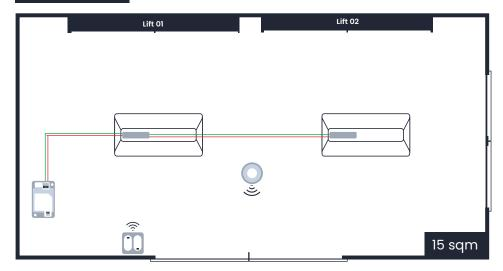
45m is the device-to-device BLE communication distance with LoS. Actual range depends on the installation and varies between 10-45m
