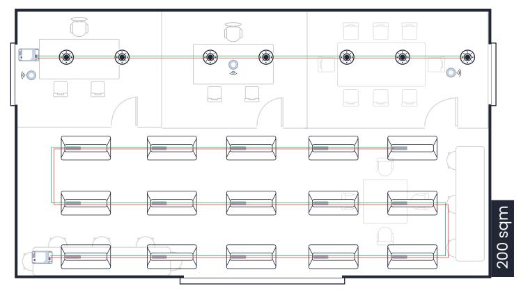
45m is the device-to-device BLE communication distance with LoS. Actual range depends on the installation and varies between 10-45m
