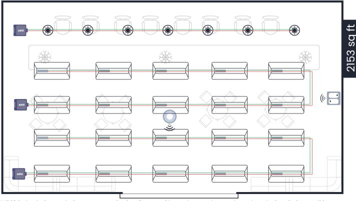
147.6ft is the device-to-device BLE communication distance with LoS. The actual range depends on the installation conditions and varies between 30ft - 130ft.
