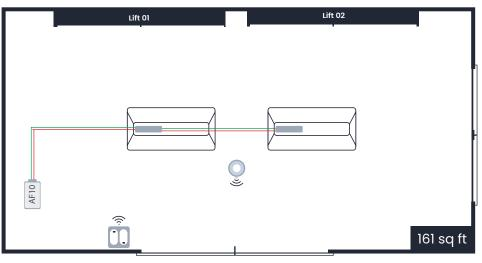
147.6ft is the device-to-device BLE communication distance with LoS. The actual range depends on the installation conditions and varies between 30ft - 130ft.
