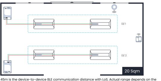
45m is the device-to-device BLE communication distance with LoS. Actual range depends on the installation and varies between 10-45m
