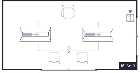
147.6ft is the device-to-device BLE communication distance with LoS. The actual range depends on the installation conditions and varies between 30ft - 130ft.
