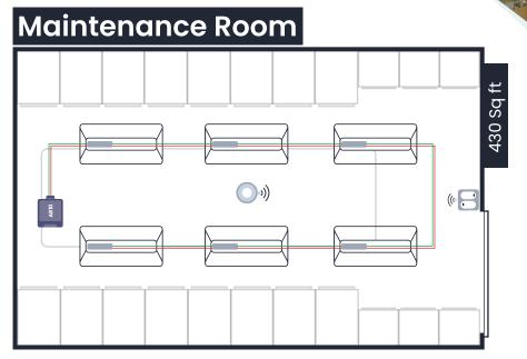
147.6ft is the device-to-device BLE communication distance with LoS. The actual range depends on the installation conditions and varies between 30ft - 130ft.
