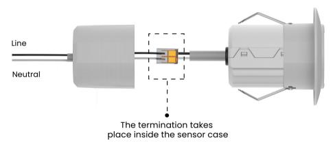
Additional junction box is not required for the sensor as the termination will happen inside the sensor case.
