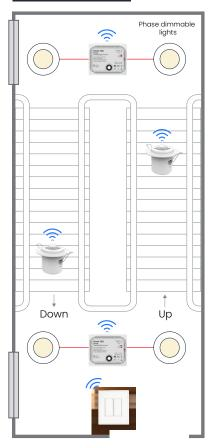
147.6ft is the device-to-device BLE communication distance with LoS. The actual range depends on the installation conditions and varies between 30ft - 130ft.
