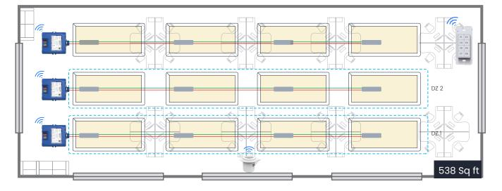
147.6ft is the device-to-device BLE communication distance with LoS. The actual range depends on the installation conditions and varies between 30ft - 130ft.
