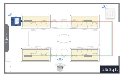
147.6ft is the device-to-device BLE communication distance with LoS. The actual range depends on the installation conditions and varies between 30ft - 130ft.
