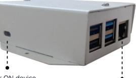
Power ON device with 5VDC Adapter
