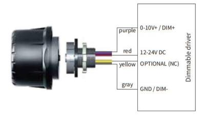
The product is powered from 12-24VDC auxiliary output of driver. 0-10V output channel is connected to the driver for dimming.
