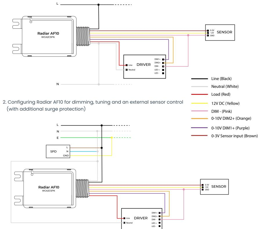
1. Configuring Radiar AF10 for dimming, tuning and an external sensor control
